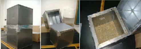
**Method A – determining the radon diffusion coefficient under non-stationary conditions**
