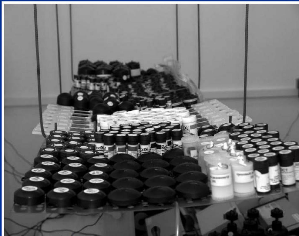
Figure 13: Detail of detectors installed in one of the rooms located in the ground floor for radon indoors passive detectors exercise
